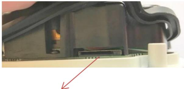
Insert the SD Card in the slot indicated by the arrow
