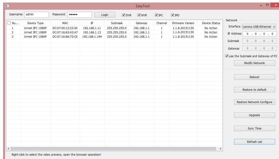
If the searched IP address and PC IP address are not in the same network segment, user may modify IP address, subnet mask, and other parameters of IP camera by using Easy Tool software.
