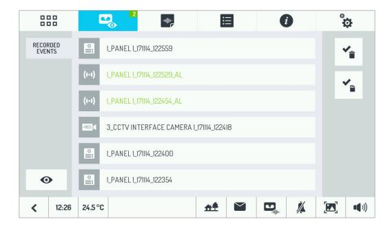
The icon on the left can be used to quickly recognise the recording type: (1) indicates a video clip saved in the event of alarm, indicates a video clip recorded from the panel using the video door phone function or manually during a call, the icon indicates a video clip recorded by additional camera.
