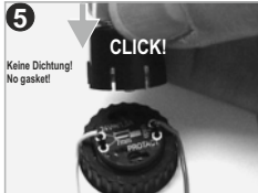
LED-Einheit festclippen Fix the LED unit
