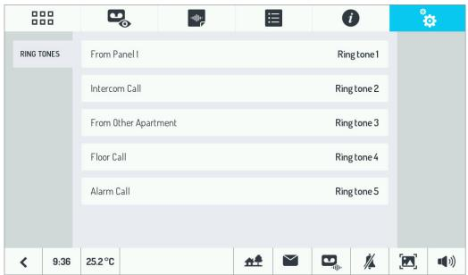
From this page it is possible to select a melody (from among the 5 proposed) for the calls from an external door unit, intercom calls from other video door phones installed in the same apartment, intercom calls from video door phones in the adjacent apartment, floor call, and the alarm signal.
