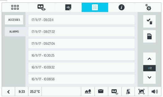
Touch the icon with the symbol of the microSD card to the top right: saving will be started. During saving, the icon will turn blue, usually for a very short time.
