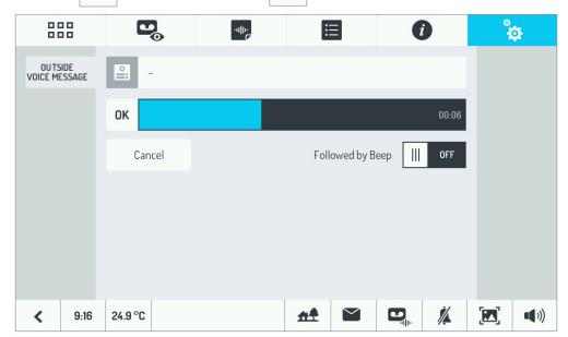
The maximum length of a message is 20 seconds. The recording may be interrupted sooner by touching the icon.
