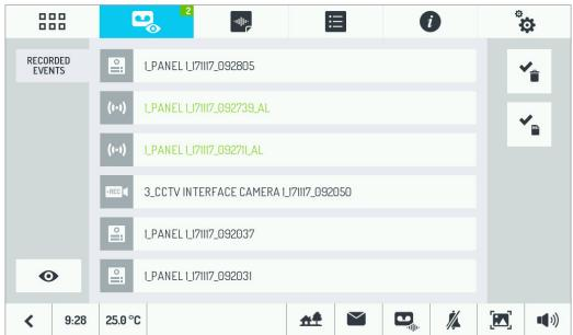
The icon on the left facilitates the type of recording: (i-i) indicates a videoclip saved in case of an alarm, indicates a videoclip recorded by an external door unit via the video door phone answering device or manually during a call, the icon indicates a videoclip recorded by an additional camera.
