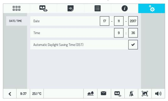
When entering the date and time, it is necessary to FIRST cancel the contents of the field and THEN insert the new value desired. To move from one field to another, touch the desired field.
