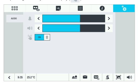
If the user should decide to silence the ring tone of the video door phone, for example while sleeping, it is sufficient to touch the soft touch the soft touch below. To reactivate the ring tone, touch the button again.
