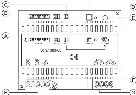
**A** - User code dip-switch used to identify the decoder in the system
