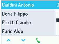
The buttons can be used to scroll the names. Hold pressed for longer than 1 second for fast scrolling.
