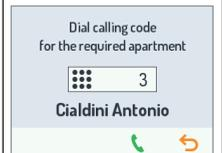
The message shown by the side will appear and a voice message will be heard if the line is busy or the apartment station is being used in another conversation. "THE LINE IS BUSY." Furthermore, the LED corresponding to the symbol (present on the front panel of the module) will light up in red on the audio or audio-video door unit.
